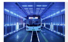
The Shanghai public transport company has converted a washing station by integrating 120 UV lamps to disinfect its buses. This new process allows them to reduce the decontamination time from 40 minutes to 5 minutes.
