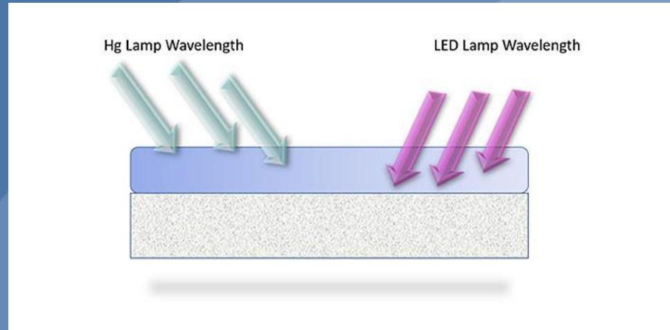
It is well noted that the longer wavelengths can suffer from poorer surface cure without an optimized formulation. There can be the same percentage of cure overall but to feel the LED coating will appear "less cured" this is not actually the case, but the surface is less cross linked so gives a softer feel than if cured under a mercury lamp.
