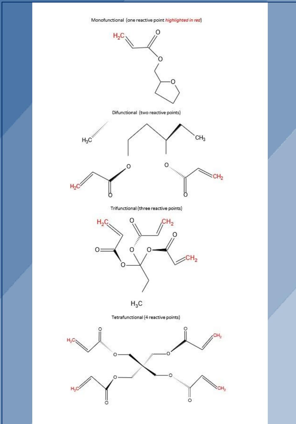
Like coiled springs these molecules are primed to react with the slightest amount of encouragement. When this happens the liquid solidifies into a gelled mass or a rock hard plastic, dependent on the type of reactivity the molecules have or the degree to which they have reacted.
